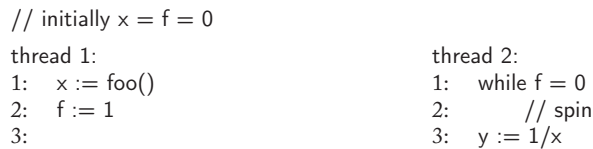
Figure 2.5: A simple example of flag-based synchronization. To avoid a spurious error, the update to x must be visible to thread 2 before the update to f .
